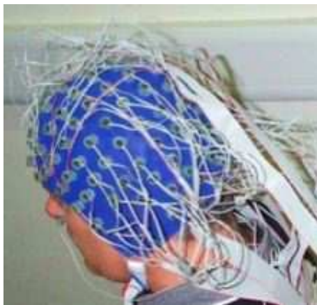
Figure 2: The 10-20 configuration is the most common to obtain EEG data for diagnosis. The number of electrodes depends on the equipment available and the required precision.
