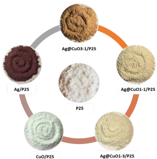
Figure 3. Pictures of the modified \text{TiO}_2 with Ag, CuO and Ag@CuO clusters (with different Ag/Cu ratios).
