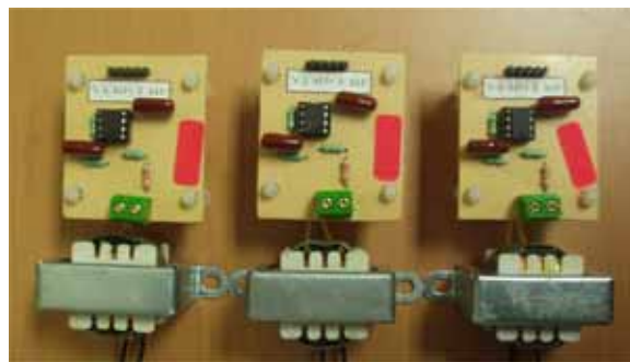
Fig. 4.9: Electric circuit of the capacitor voltage sensor.
